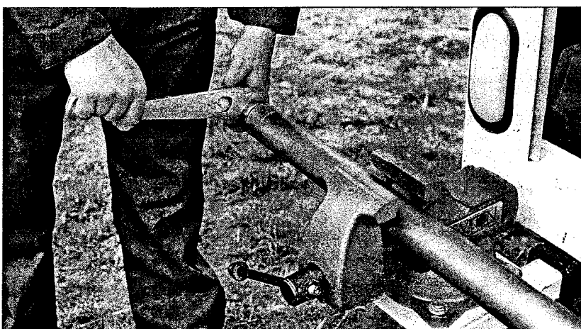
Figure 4.9. Tighten MC Drive Head with MC Combination Wrench. A vise is often used to hold the MC Sample Tube during this step.
