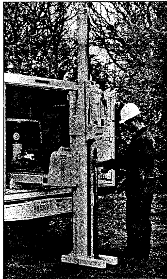
Figure 4.24 MC Sampler positioned for driving into subsurface.
